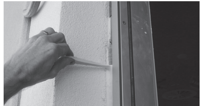
FIGURE 6.6 – FIELD ADHESION TEST
